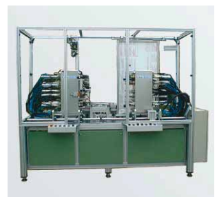
23 placing heads to assemble a computer chassis
